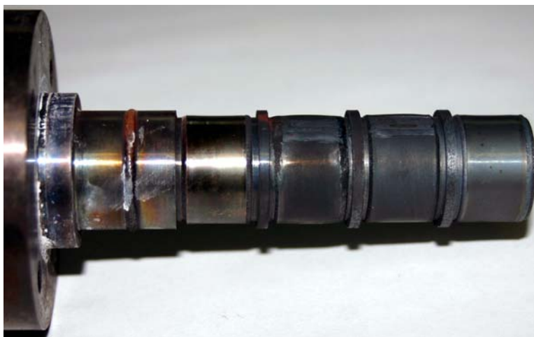
Figure 2. Sample holder after 500-hr exposure in ORNL's microturbine recuperator test facility. From left to right, the foils that were evaluated are: alloy LCF-625, ORNL-modified stainless steel, ORNL-modified stainless steel, and alloy LCF-625.
