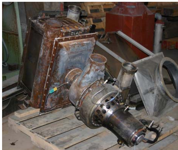
Figure 5. Recuperator box removed from Bowman microturbine.
