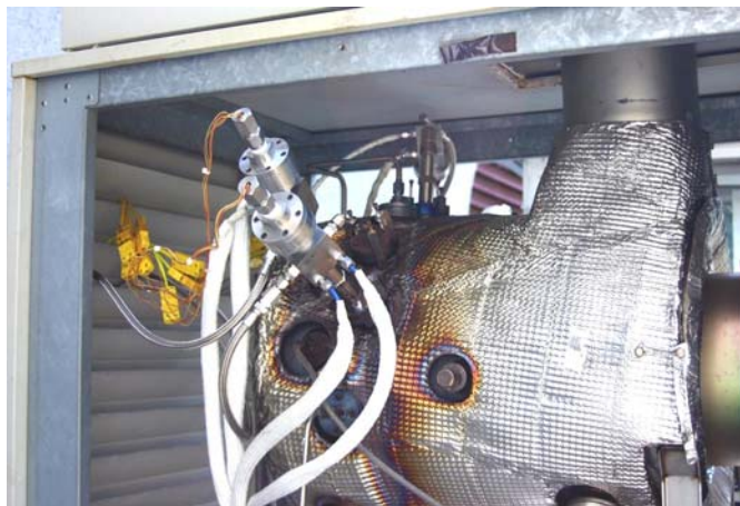
Figure 1. Photograph of ORNL's microturbine recuperator test facility operating with four sample holders.
