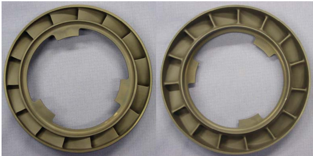
Figure 1. Photos of UTRC SN282 silicon nitride integral vane ring designed for ST5+ advanced microturbine system.
