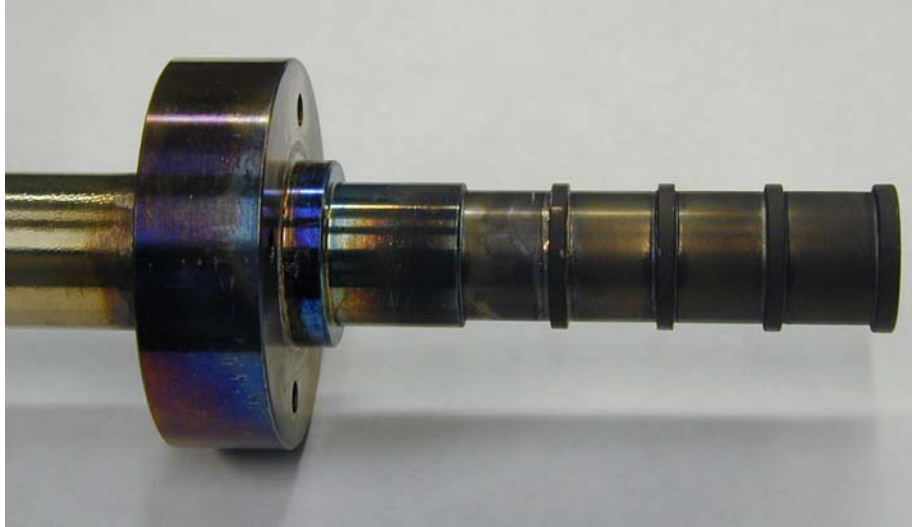
Figure 4. Photographs of sample holder with 0.089-mm thick Haynes 120® foils after 500-hr test at TET=800°C and internal pressure of 60 psi.
