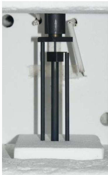
Figure 5. Close-up view of the specimen, loading and support rods, and transducer rods inside the furnace.
