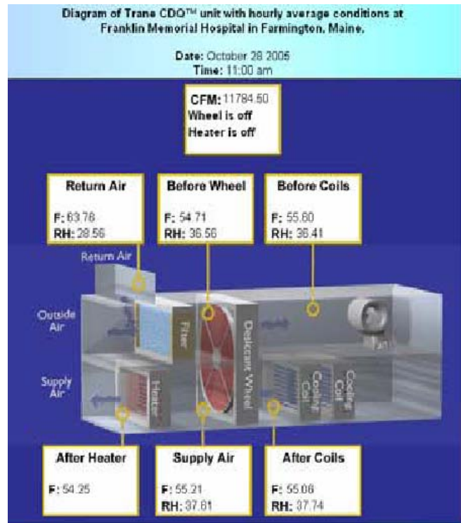
Figure 5: Graphic Schematic of the Franklin Memorial Hospital CDQ™ desiccant installation continuously available on the internet
