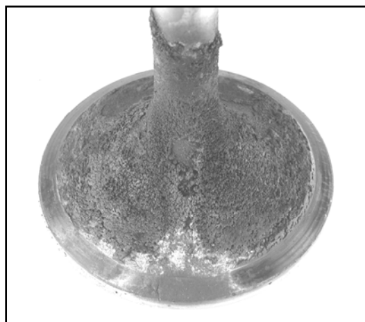
Figure 1. Overall view of a torched intake valve (7000 h engine test) showing the partial spallation of a heavy oil deposit.
