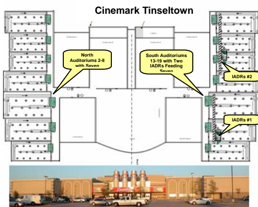
Figure 1: CineMark Tinseltown theater showing side-by-side installation of SEMCO IADR units and conventional rooftop units for field trial test.
