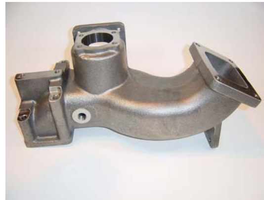
Figure 4 – A CF8C-Plus cast stainless steel exhaust component for a Waukesha natural gas reciprocating engine made by Stainless Foundry & Engineering. This component is the bridging structure between the exhaust manifolds and the turbocharger.
