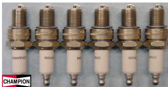
Figure 4 Photo shows the conventional J-type natural gas engine spark plugs incorporating ORNL developmental alloys.
