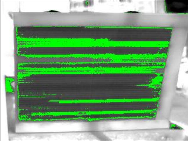
Figure 2 Flow maldistribution shown with thermal imaging camera
