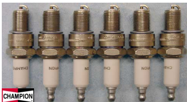
Figure 6 Photo shows the conventional J-type natural gas engine spark plugs incorporating ORNL developmental alloys.
