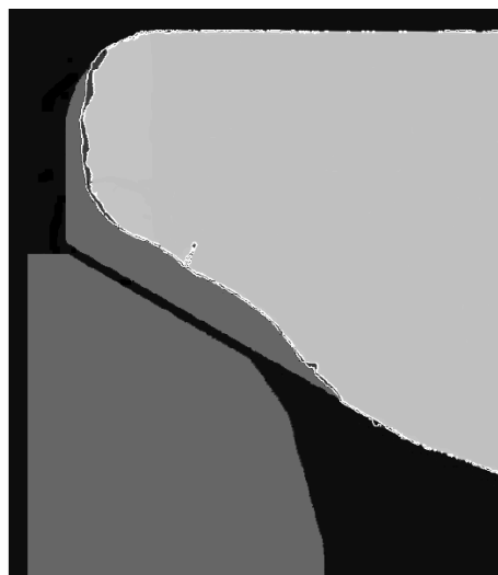
Figure 2. Cross section of a torched valve (7000 h) showing about 1 mm metal recession due to erosion, oil deposits, metal oxidation and surface cracking. The degree of recession is shown by the original (dark gray) profile.
