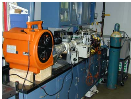
Figure 7. Retrofitted Test Rig with Blower Assembly
