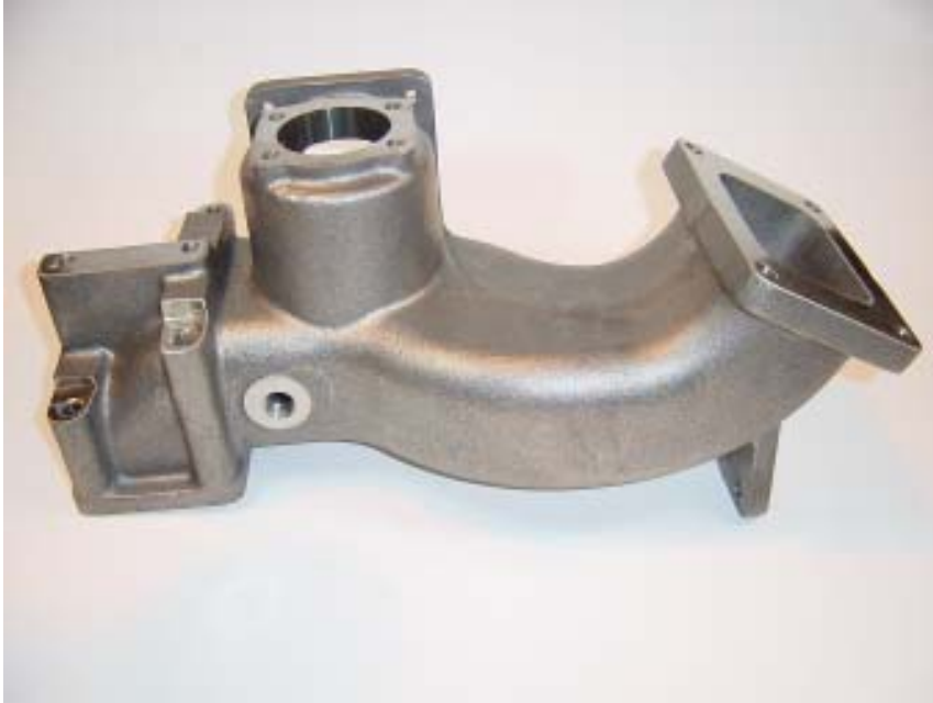
Figure 1 – First successful cast trial of an exhaust component made from the new CF8C-Plus cast stainless steel by Stainless Foundry and Engineering, Inc. for Waukesha Engine Dresser, Inc.
