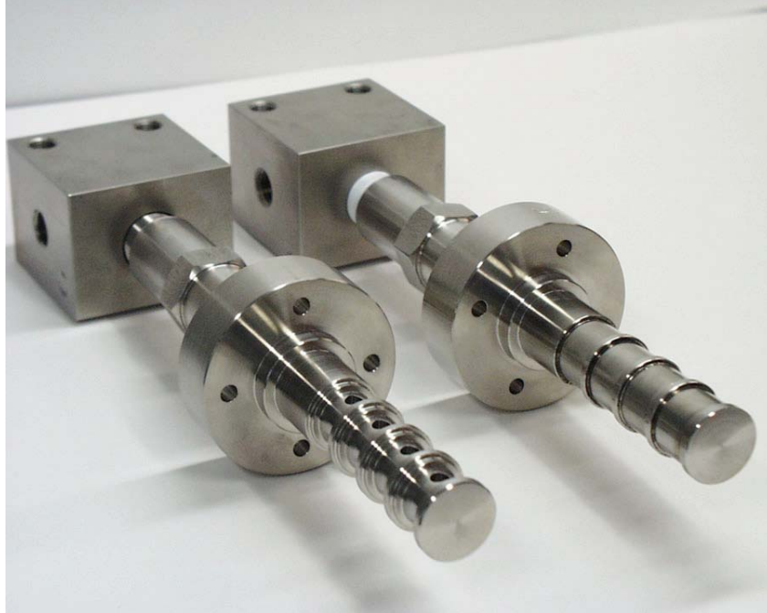
Figure 2. Sample holders for exposure of metallic foils in ORNL's microturbine recuperator testing facility. The orifices where thermocouples are placed and that are used to allow mechanical stressing of test specimens through pressurization is shown on the left. A sample holder with laser-welded metallic foils is shown on the right.
