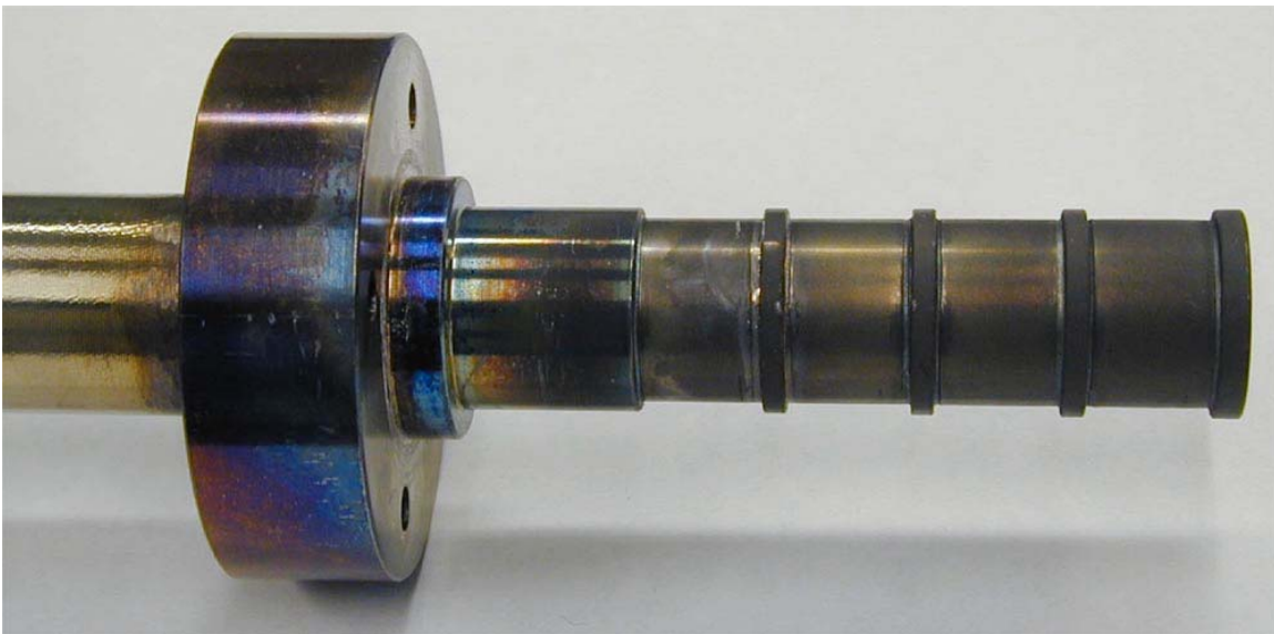
Figure 11. Sample holder with HR120® alloy foils after 500-hr exposure in ORNL's microturbine recuperator testing facility at TET=800°C.
