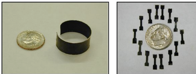
Figure 10. Foil after being removed from sample holder at end of 500-hr exposure test. Fourteen miniature tensile specimens were obtained from each foil.
