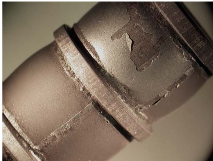
Figure 9. Optical micrograph of foils A and B (0.089-mm thick foils of 347 stainless steel), after 500-hr test at a TET of 800°C and tensile tangential stress of 50 MPa. Note the corrosion scale on the surface of the foils. The weld seam in foil B is evident.
