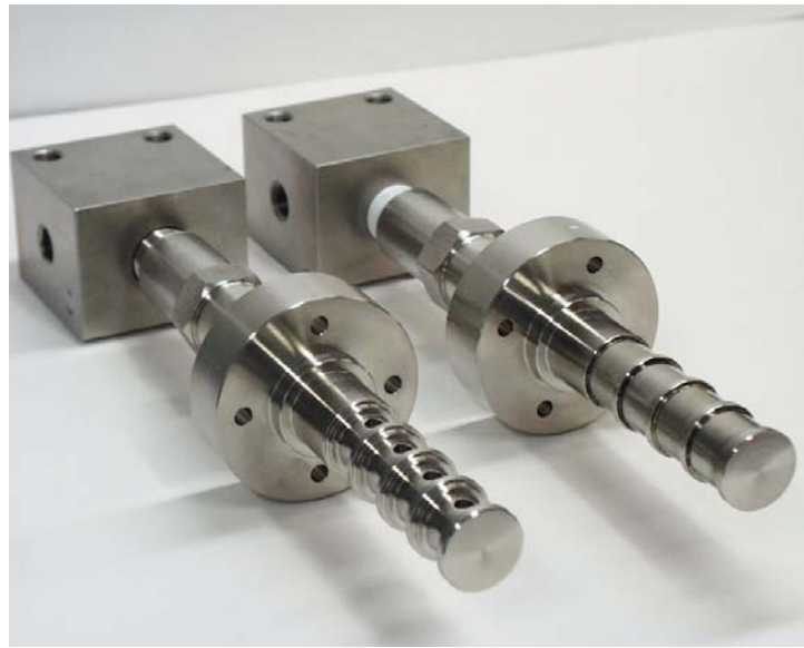
Figure 2. Sample holders with and without foils. The holes in the sample holder allow the placement of thermocouples and the flow of gas for mechanically stressing the foils through the internal pressurization of the sample holder.
