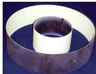
CFCC combustor liners with EBC on gas-path surfaces
