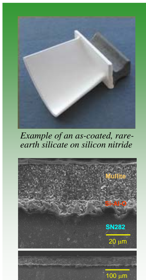
Micrographs of polished cross-sections of densified mullite on silicon nitride
