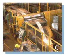
*The AL20-25+Nb stainless alloy* was melted as a large ingot. It was then formed into foils and sheets through typical commercial rolling of hot-band (A), cold-rolling and annealing (B), and slitting to the exact widths required by each recuperator manufacturer (C).
