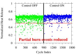
In this example, application of adaptive control to a small NG engine operating at lean conditions results in a 70-75% reduction in the occurrence of extreme partial burns and misfires.
