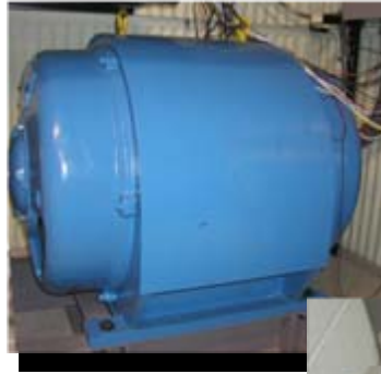
250 kVar synchronous motor & 75, 150 & 300 kVar 3-phase inverters
