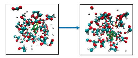
Spontaneous solvation of LiPF<sub>6</sub> salt in ethylene carbonate revealed by first principles molecular dynamics simulations
