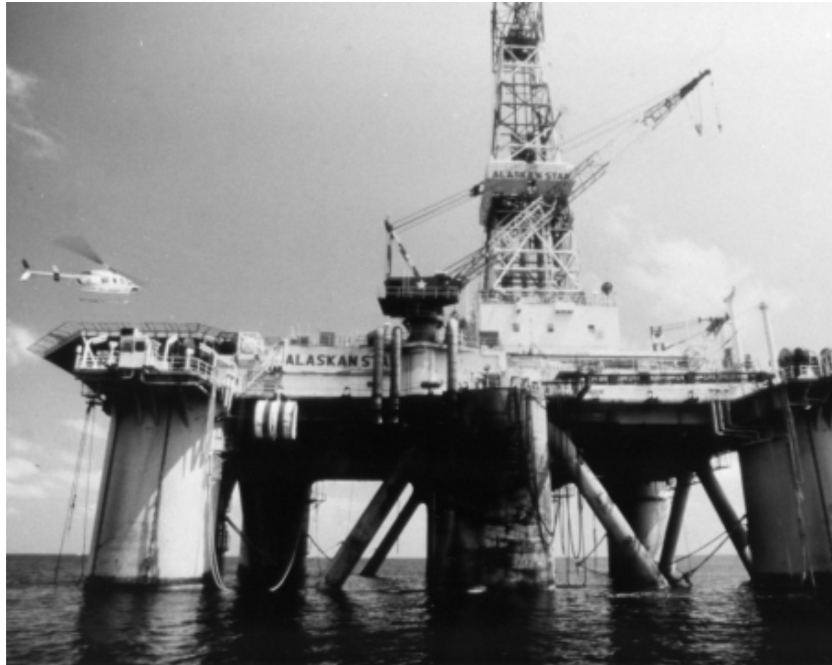
Semisubmersible drilling rig in the Gulf of Mexico. Source: U.S. Department of Energy.
