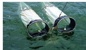
A standard 61-cm bongo net fitted with 0.333-mm mesh used in plankton sampling.
