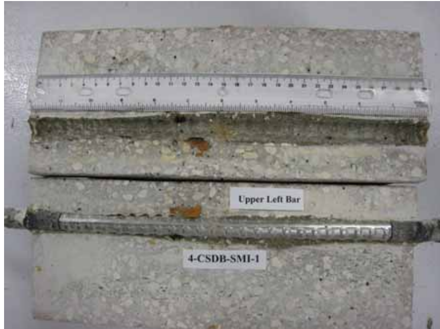
Figure 98. Photo. Top L bar and bar trace of specimen 4-CSDB-SMI-1 subsequent to dissection.
