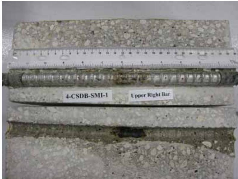
Figure 97. Photo. Top R bar and bar trace of specimen 4-CSDB-SMI-1 subsequent to dissection.
