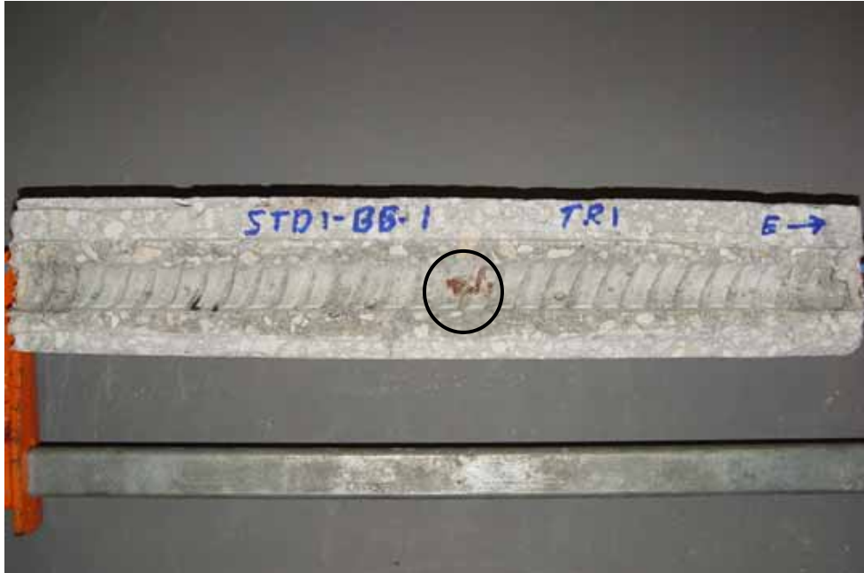
Figure 86. Photo. Upper R bar trace of dissected specimen 5-STD1-BB-1 showing localized corrosion products (circled).
