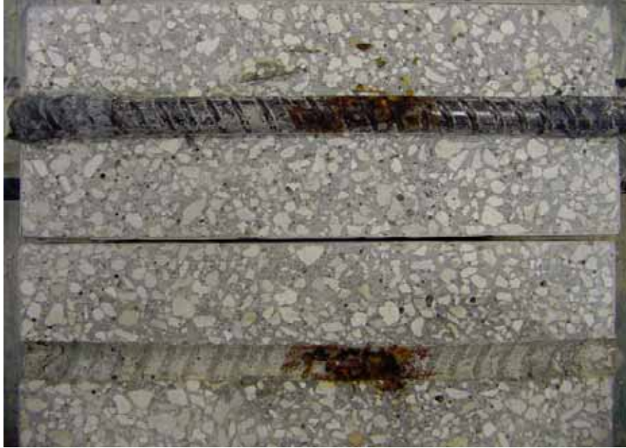
Figure 107. Photo. Top bar and bar trace for specimen MS-MMFX-2-C.
