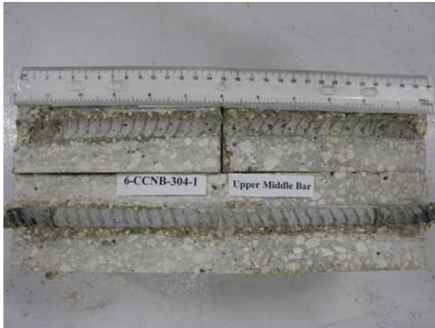
Figure 102. Photo. Top C bar and bar trace of specimen 6-CCNB-304-1 subsequent to dissection.
