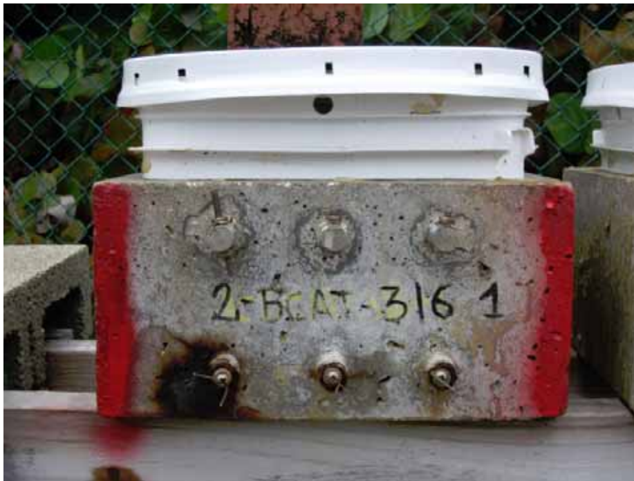
Figure 88. Photo. Specimen 2-BCAT-316-1 prior to dissection (red markings identify specimen for removal).
