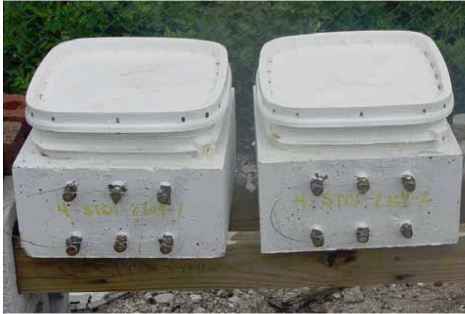
Figure 10. Photo. Two SDS specimens under exposure.
