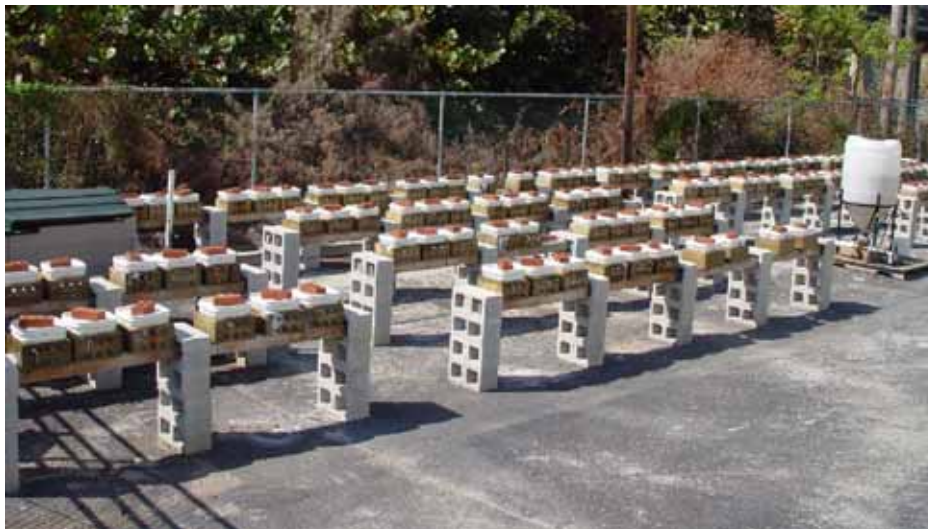
Figure 11. Photo. SDS specimens under exposure in the outdoor test yard.
