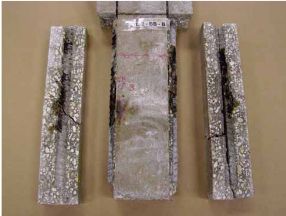
Figure 114. Photo. Specimen 3BTC-STD2-BB-B after sectioning and opening along the two longer bars.
