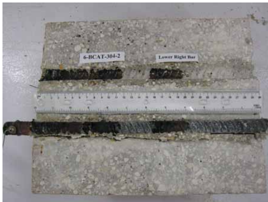
Figure 101. Photo. Lower right BB and bar trace of specimen 6-BCAT-304-2 subsequent to dissection.
