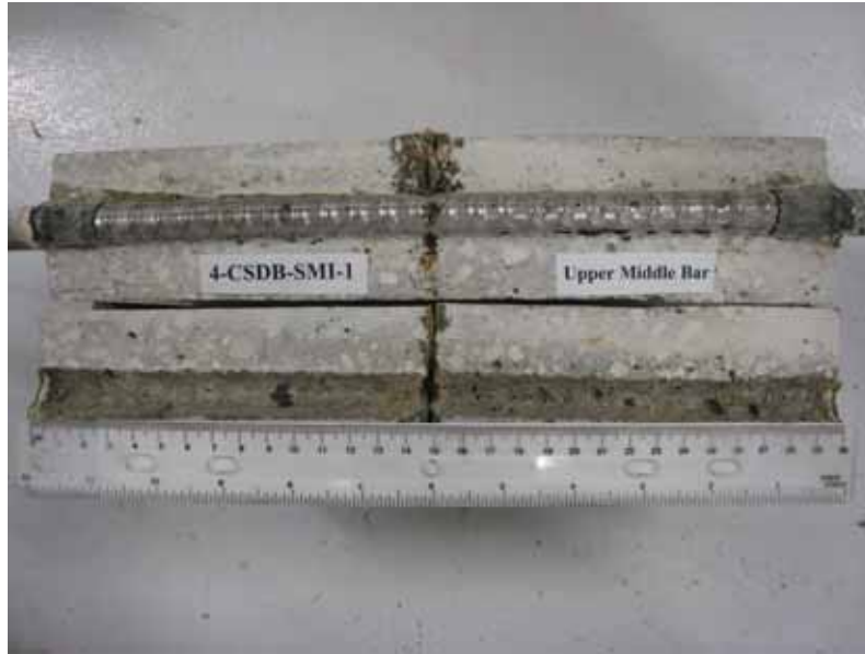
Figure 96. Photo. Top C bar and bar trace of specimen 4-CSDB-SMI-1 subsequent to dissection.
