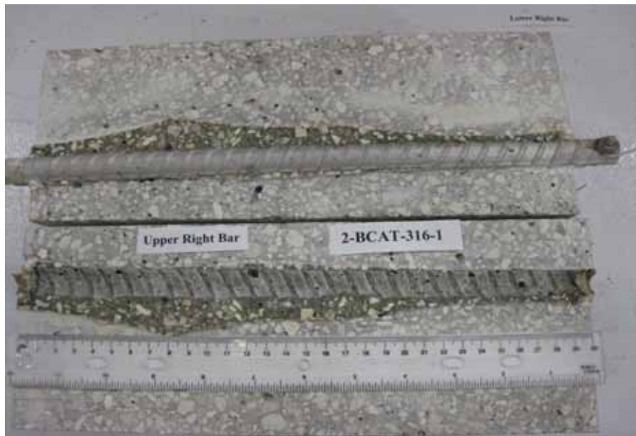
Figure 89. Photo. Top R bar and bar trace of specimen 2-BCAT-316-1 subsequent to dissection.
