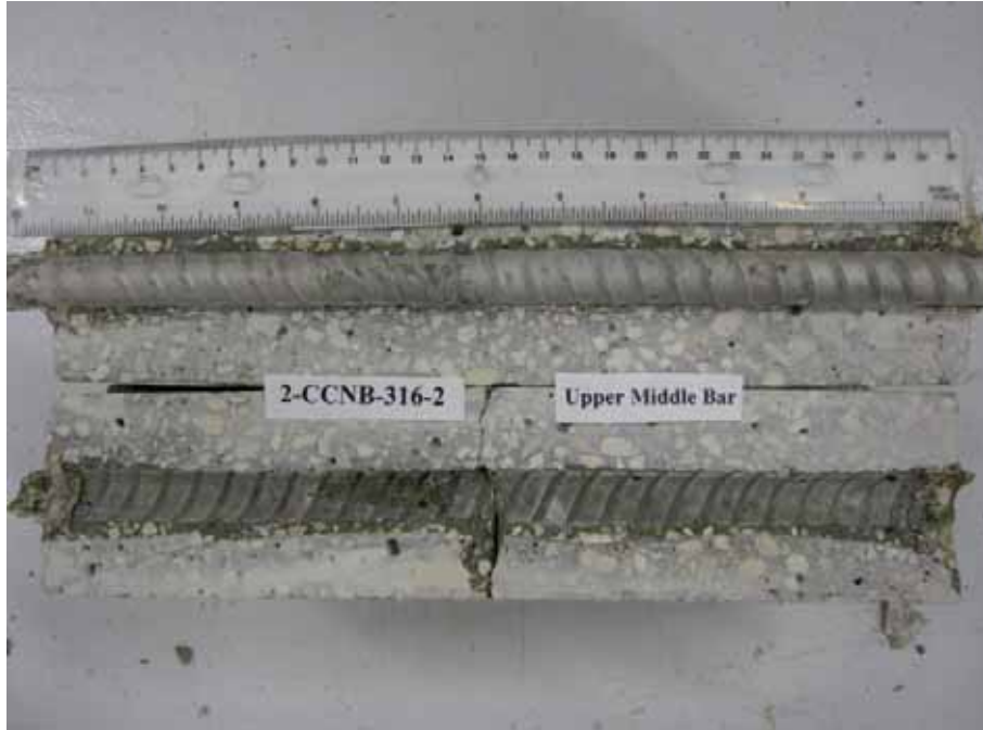
Figure 92. Photo. Top C bar and bar trace of specimen 2-CCNB-316-2 subsequent to dissection.
