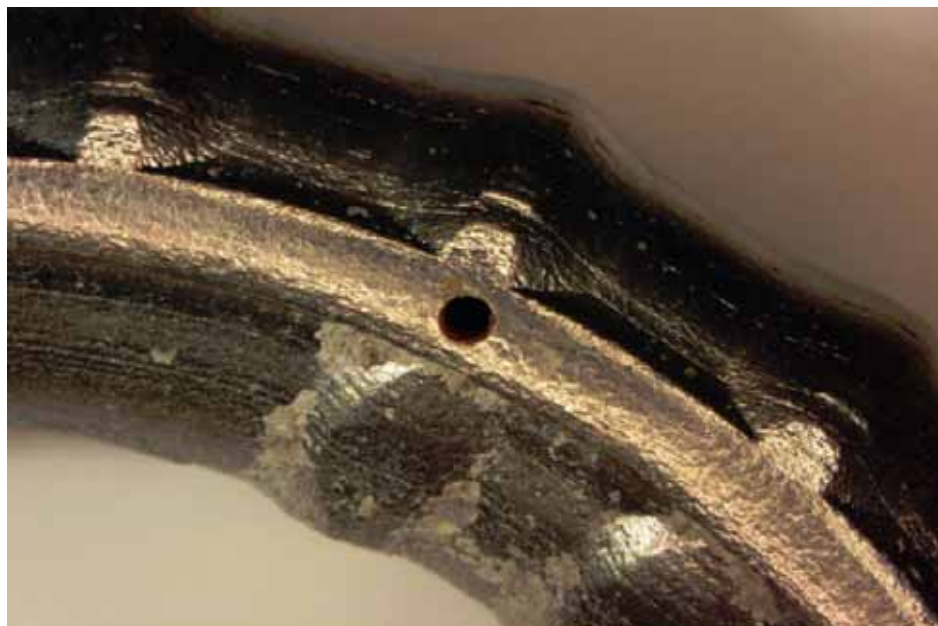
Figure 113. Photo. Corrosion at a second intentional clad defect on the top bent bar from specimen MS-CBDB-SMI-B.
