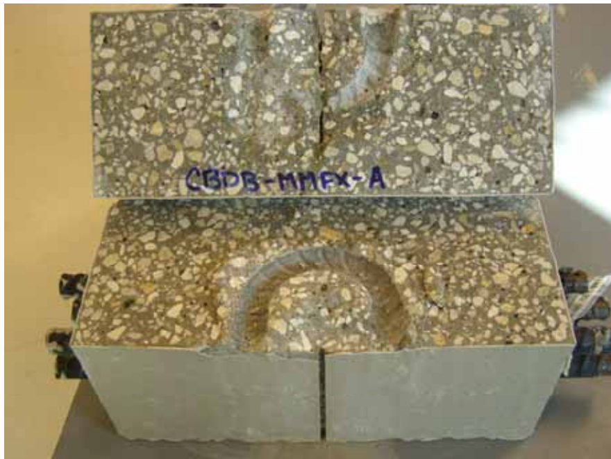
Figure 108. Photo. Top bent bar trace in concrete for specimen MS-CBDB-MMFX-2-A.
