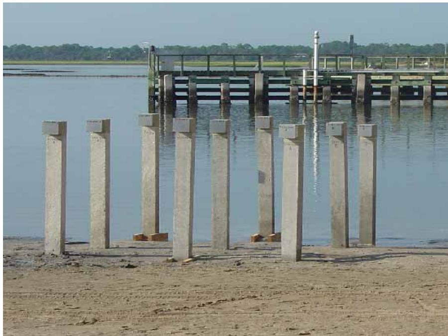
Figure 20. Photo. Field column specimens under exposure at the Intracoastal Waterway site in Crescent Beach, FL.
