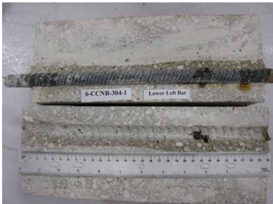
Figure 103. Photo. Lower left BB and bar trace of specimen 6-CCNB-304-1 subsequent to dissection.
