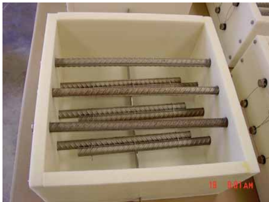
Figure 9. Photo. View of a mold for a CCRV-SMI specimen prior to concrete pouring.
