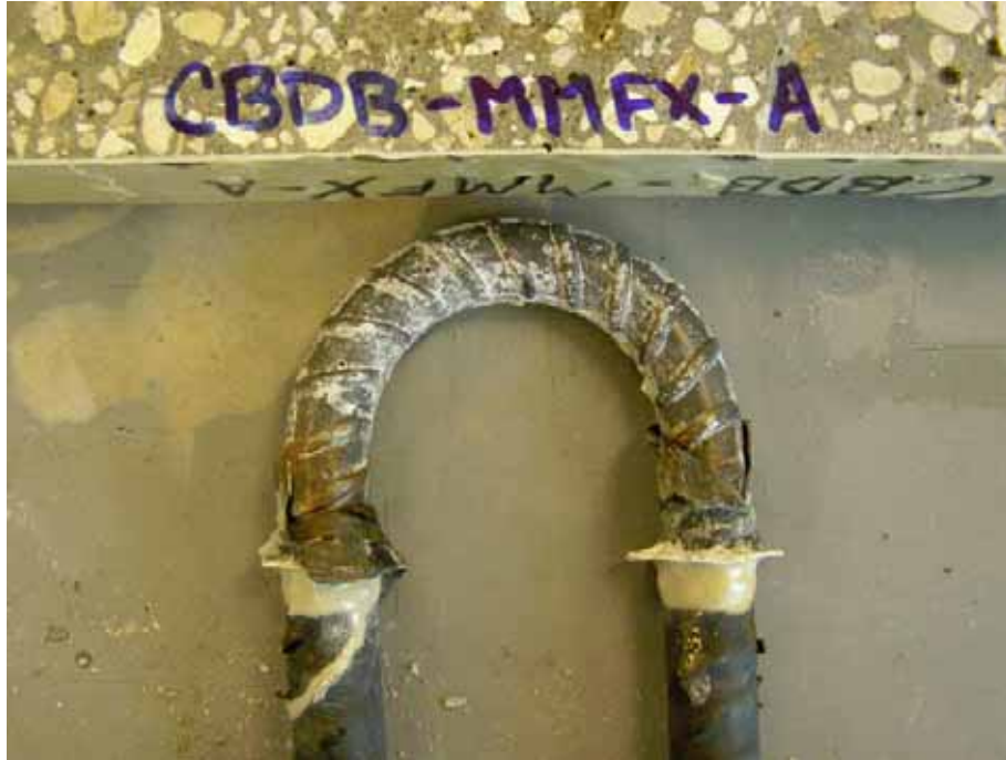
Figure 109. Photo. Top bent bar from specimen MS-CBDB-MMFX-2-C after removal.
