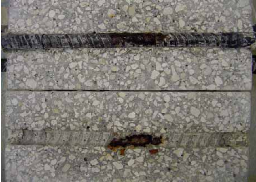
Figure 105. Photo. Top bar and bar trace for specimen MS-MMFX-2-A.
