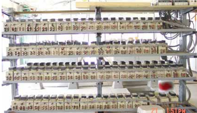
Figure 14. Photo. MS slab specimens under exposure.
