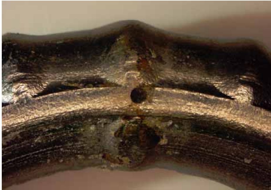
Figure 112. Photo. Corrosion at an intentional clad defect on the top bent bar from specimen MS-CBDB-SMI-B.
