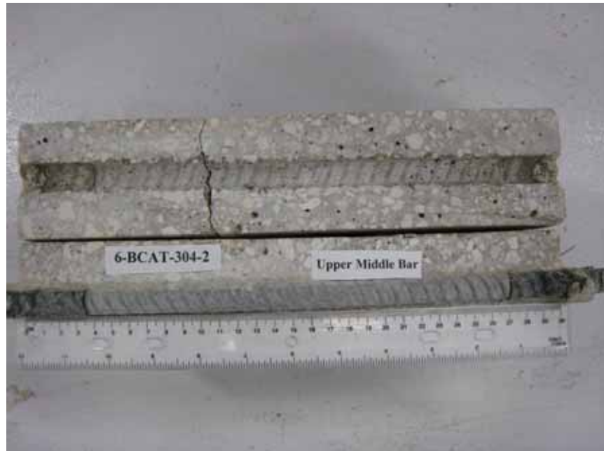
Figure 100. Photo. Top C bar and bar trace of specimen 6-BCAT-304-2 subsequent to dissection.
