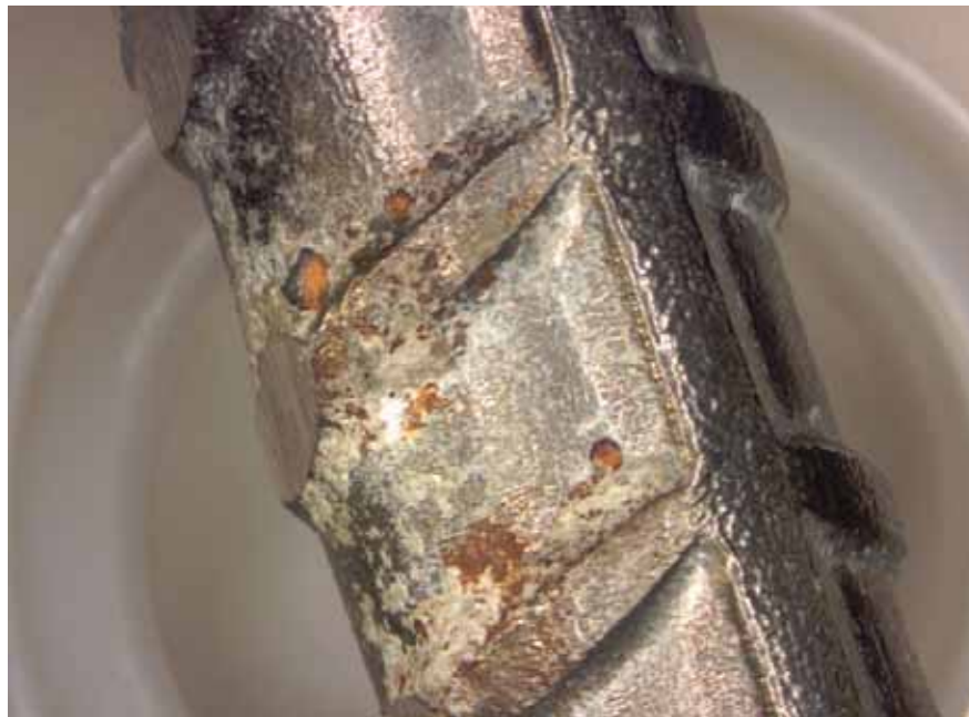
Figure 111. Photo. Localized corrosion on the top bent bar from specimen MS-CBNB-316-B.
