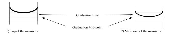
When opaque liquids are used, an additional error or correction factor can be estimated based on the volume contained between the upper and lower edges of the meniscus. The curve of the meniscus and impact of this error is dependent on the diameter of the meniscus and surface tension of the liquid being used.
