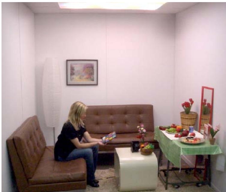
Figure 5. The Division’s Spectrally Tunable Lighting Facility consists of two room-size, furnished cubicles in which observers can be completely immersed in a real-life setting. Each cubicle is lit by 1,800 variable-power LEDs under computer control. The LEDs span the visible spectral range and can be set to simulate the spectra of various types of light sources for testing and optimizing using vision-science methods.
