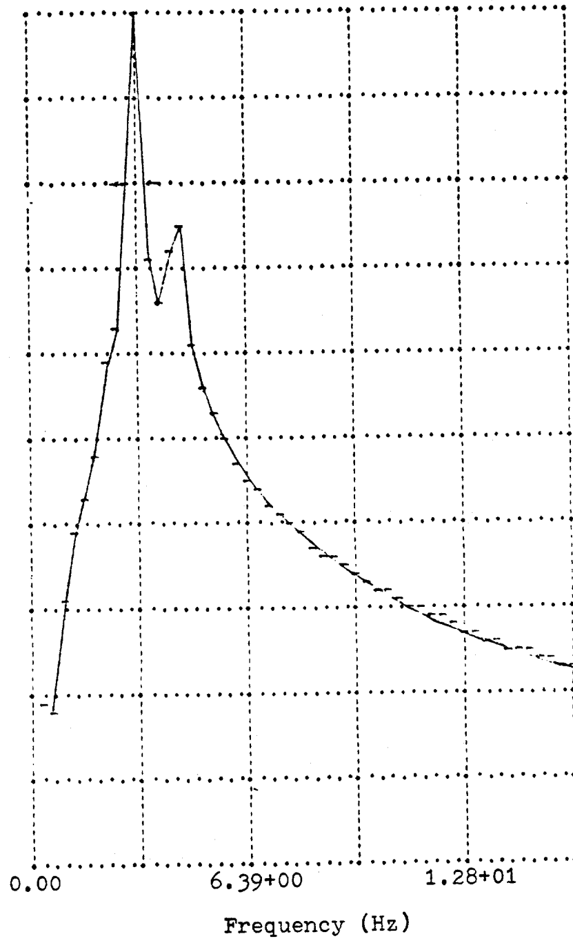
Figure 14. Power Spectral Density Curve of the Random Decrement Signature of Model C
