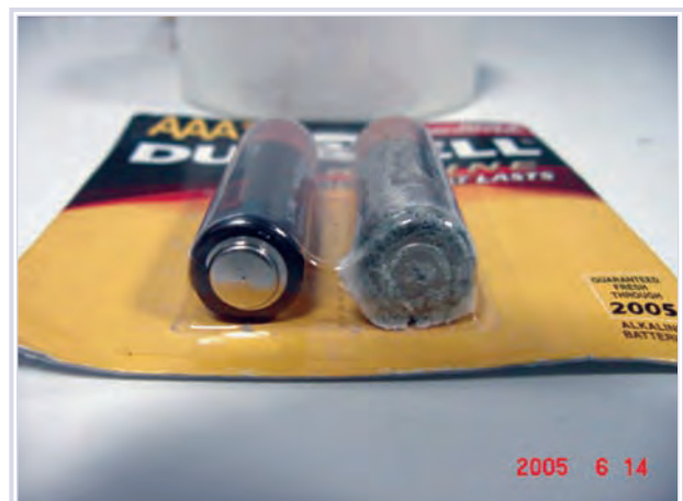
Corroded counterfeit batteries seized in Los Angeles, California by Special Agents of the United States Immigration and Customs Enforcement agency in June 2005. Photo by Dept. of Homeland Security, Immigration and Customs Enforcement.
