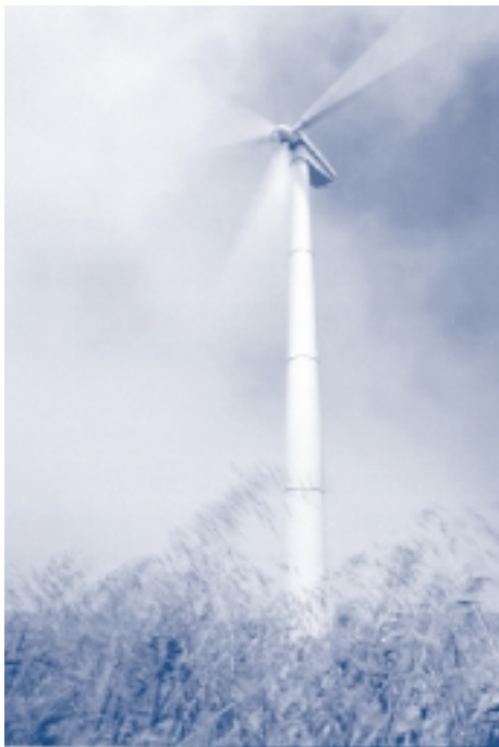
One of three 225-kilowatt wind turbines generates electricity for the Navy on San Clemente Island off the coast of California.
