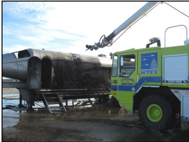
The Mobile ARFF Trainer operated by the University of Missouri Fire Rescue Training Institute has the capability to provide HRET/SPN training.
