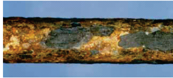
b) Pitting with Localized Exfoliation of Iron Oxide
