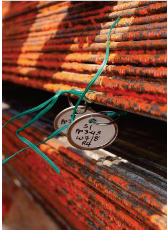
Figure 11-2 Photo showing the sample tag in wedge #7, wedge #8 side, ring #4, panel point 3-4
