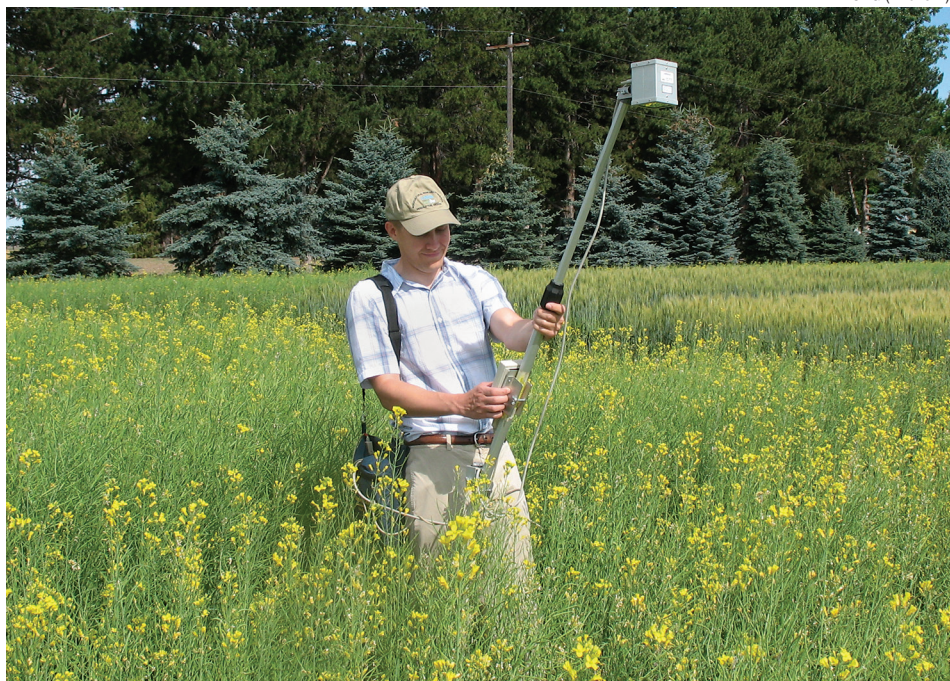
Physical research scientist John Sulik uses a hand-held radiometer to measure spectral reflectance from spring rapeseed in plots near Pendleton, Oregon. Spectral reflectance obtained with ground- and satellite-based sensors is being tested as a tool for predicting the crop’s nitrogen status, which may prove useful for predicting final oilseed traits desired by crushers and biorefiners.
