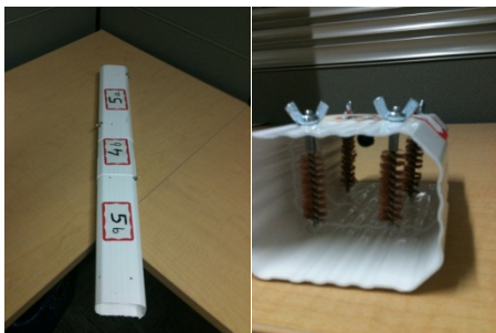
Fig.1- Gutter device (left), middle part of the gutter device with gun brushes and the alligator clip for the bait (right).
