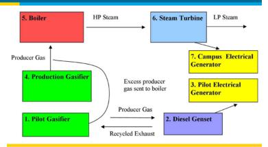
Energy-flow schematic for use of a producer gas-powered genset.
