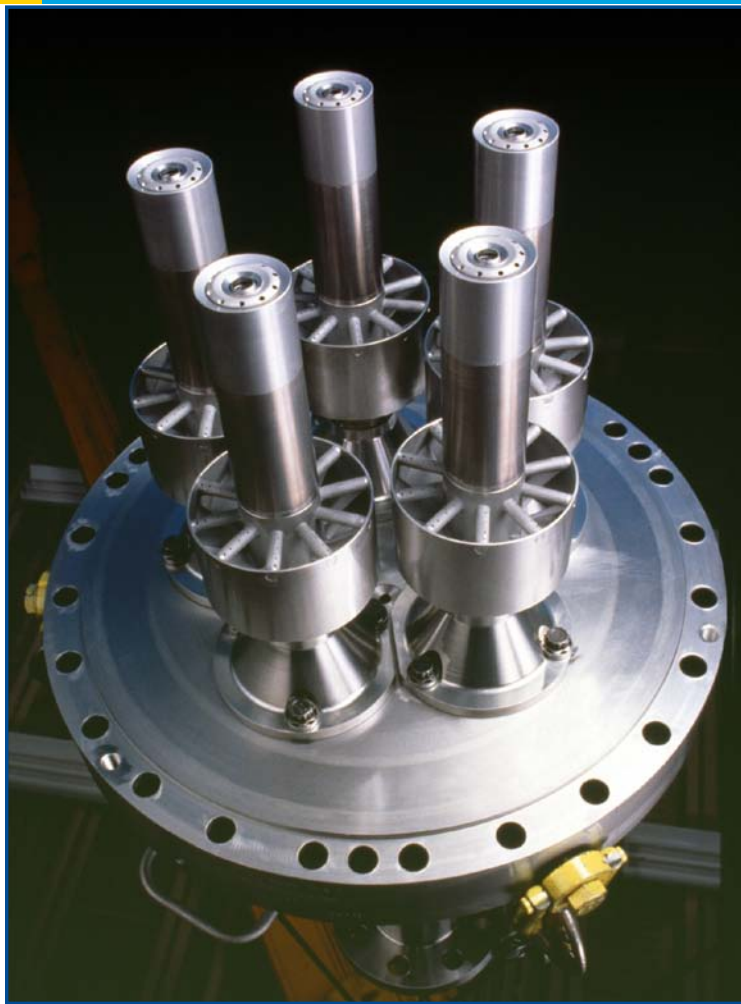
Figure 1. A Dry-Low NO x combustor end cover and premixing fuel nozzles. Evolutionary and revolutionary concepts will be evaluated in order to increase the fuel flexibility of gas turbine combustion systems.
