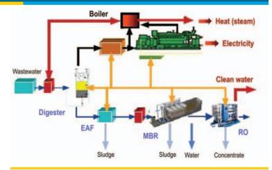
Waste-to-value plant recovers energy through anaerobic digestion and purifies the water to desired purity for reuse, moving through filtration, an aerobic membrane bioreactor (MBR), and reverse osmosis (RO). Predictive monitoring and supervisory controls are key to achieving the robust and flexible operation of the integrated plant.
