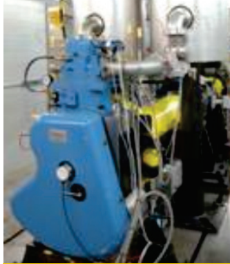
Fig 4. Argonne's nitrogen enrichment tests on a single cylinder research engine.
