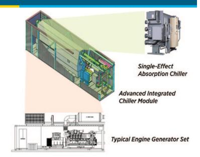
Conceptualization of Heat Recovery Absorption Chiller Module/CHP Solution
