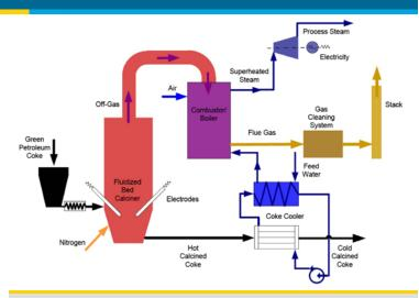
Flow chart of the petroleum coke calcining process in an electrothermal fluidized bed, integrated with waste heat utilization. The calcining process is composed of the petroleum coke charger (black), fluidized bed calciner with electrodes and nitrogen supply (red), and gas cleaning system (yellow-gold). The waste heat utilization system (or advanced CHP) is composed of the combustor/boiler (purple), coke cooler (blue), and generator (blue-violet).
