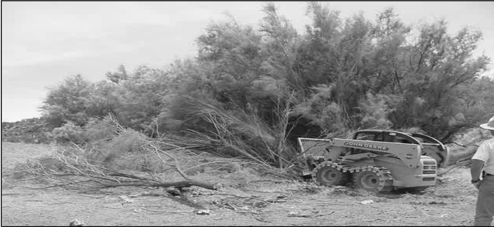
An Agroaxe is used to mechanically push Salt cedar down. The project will be followed with a prescribed fire to remove the downed vegetation.
