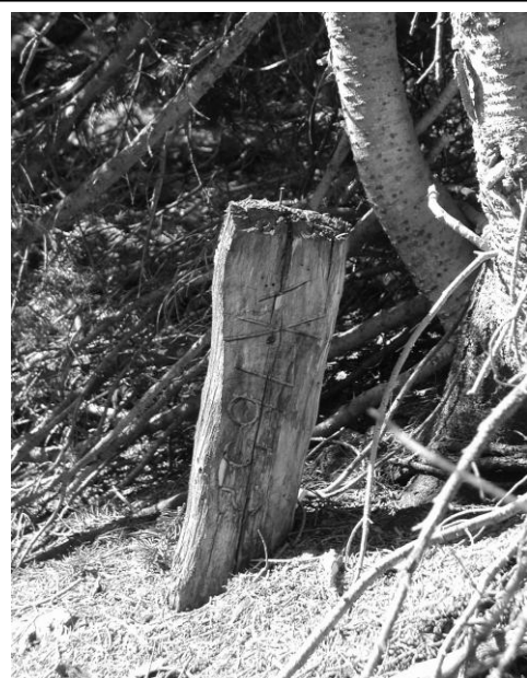
Original surveys completed in the 1800's typically have corner monumentation consisting of scribed wooden posts, such as shown here, or marked stones. Finding this original evidence is the first step in locating property boundaries of federal lands. After evidence is identified, it is replaced with modern brass-capped metal posts and properly recorded in the Federal records system -- preserving evidence for future generations.
