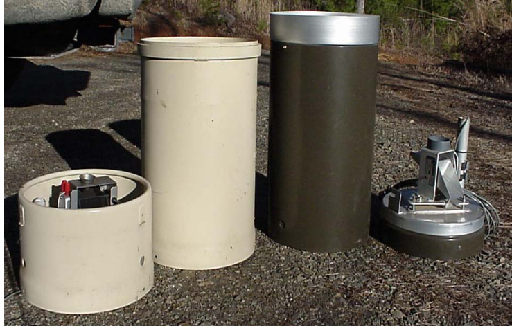
Figure F- 4. Tipping buckets and top sections for two gage brands.
