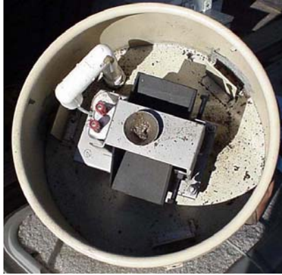
Figure F- 8. Clogged tipping bucket, top view.
