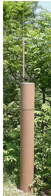
Figure 1-1. Automatic rain gage.
