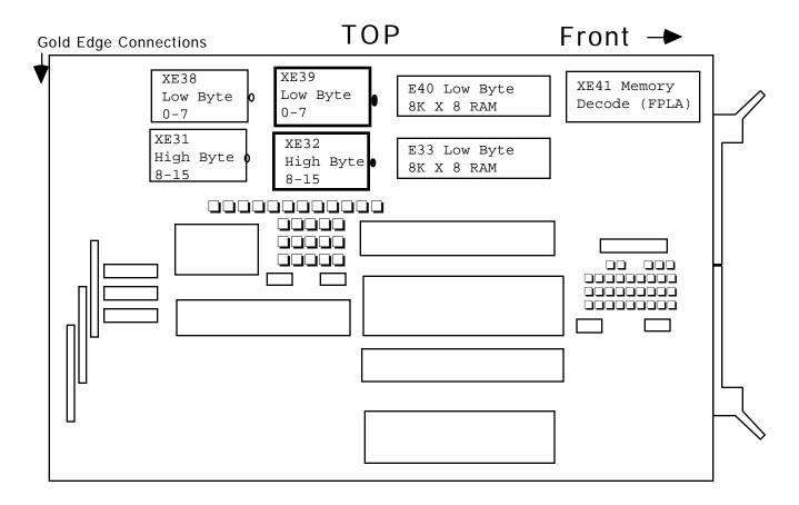
9. Orient the new chips with the chips in XE39 and XE32.
