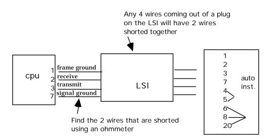
If you plug into the LSI, then check the four wires at the other end to find out which two are shorted. These are ground wires and will be connected to pins 1 and 7 (it does not matter which) on the computer port or the instrument. Now there are only two wires to worry about and they will go on 2, and 3 so if one combination does not work, try the other.
