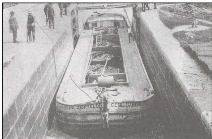
Figure 34: Canal boats were constructed for maximum carrying capacity allowed by the locks.
