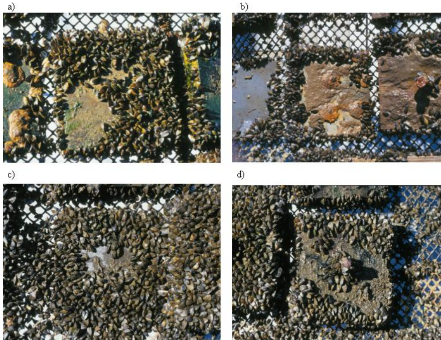
Figure 15. Examples of settlement patterns on a) soft wood from North Beach, b) steel plate from General Butler, c) PVC plate from Diamond Island, d) wood sandwich with steel post from Diamond Island.
