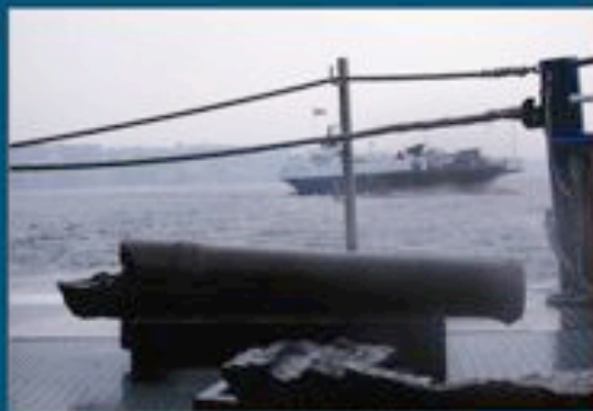
Recovered fragments of the burst cannon from the gunboat New York .
