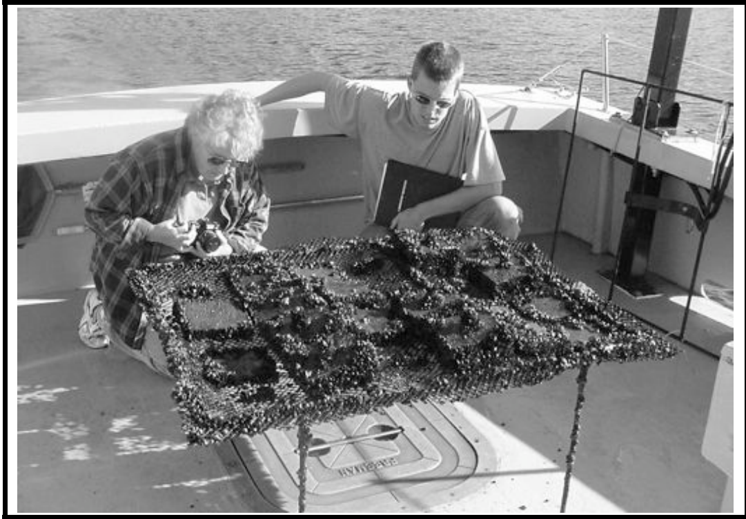
Figure 2:6. Photograph showing a zebra mussel settlement table upon recovery from Lake Champlain (Photograph by A. Cohn).
