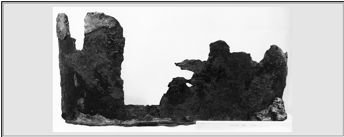
Figure 41. Section of blower housing damaged by torpedo explosion that was removed during Smithsonian project. (Naval Research Laboratory)
