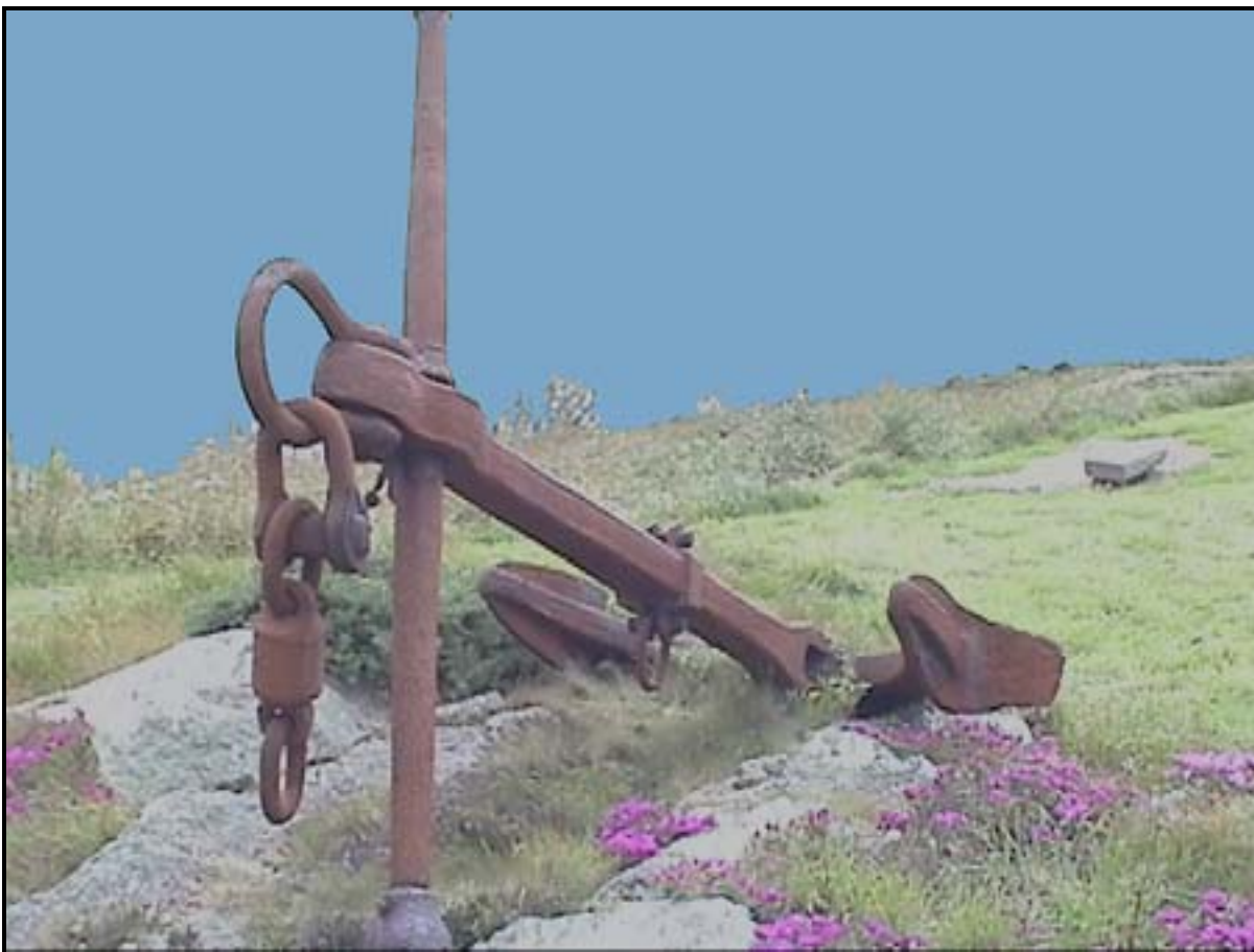
Figure 9. Example of a Trotman anchor similar to those of the CSS Alabama .
