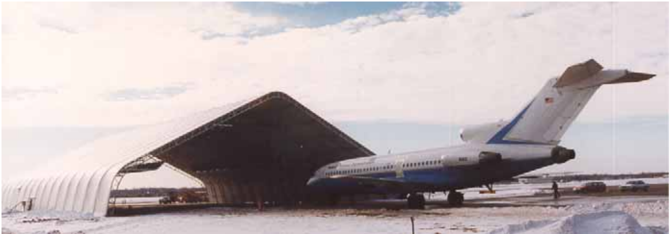
Figure 5-1. FAA Boeing 727-100 taxiing into an infra-red deicing structure
