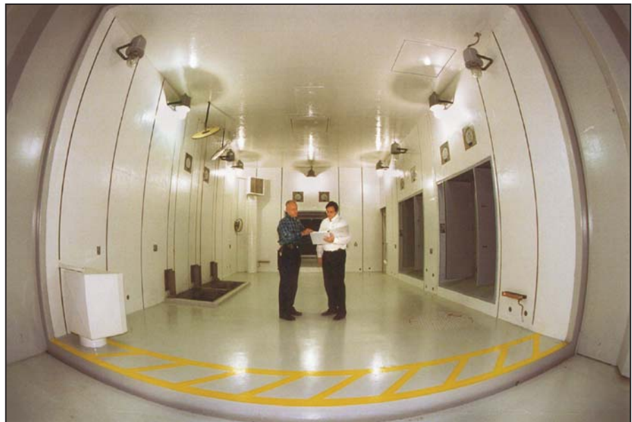
Sandia National Laboratory scientists review procedures inside the largest of the Gamma Irradiation Facility's three test cells.
