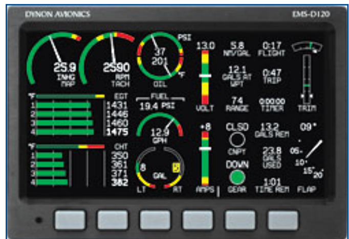
Figures 6 and 7. Dynon EMS-D120 display with engine off and engine running (Harrison and Hannon, 2009)
