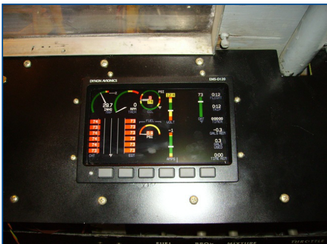
Figures 6 and 7. Dynon EMS-D120 display with engine off and engine running (Harrison and Hannon, 2009)
