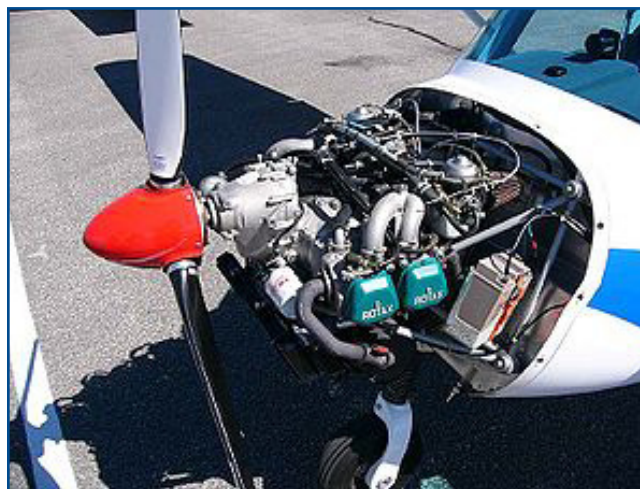
Figure 2. Typical Rotax 912 Installation
