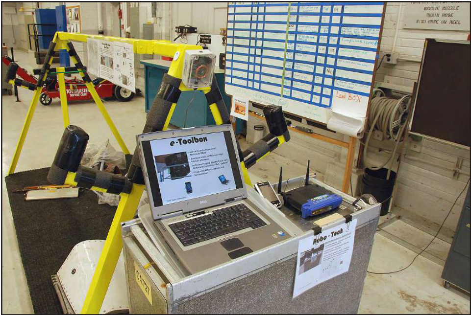
Figure 3. "Smart Cart" prototype aircraft maintenance stand
