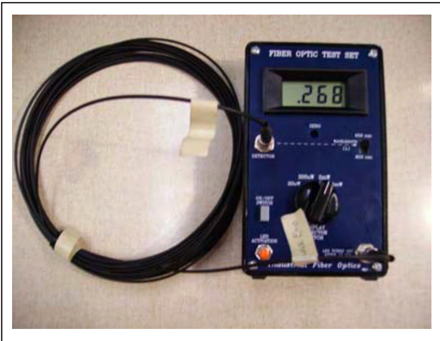
Figure 2. Fiber optic test set with cable
