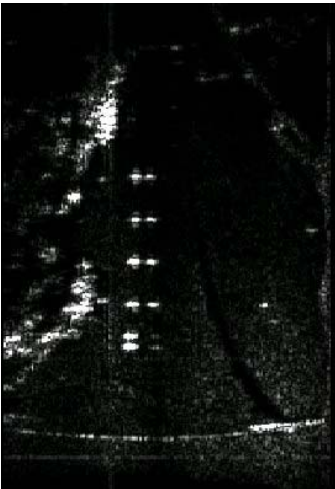
Figure 6. Radar image of the "Radar-VASI" system. The aircraft is below glide slope, because only the left pair of Diplanes with \alpha=2.3^\circ and \alpha=2.9^\circ have high intensities.
