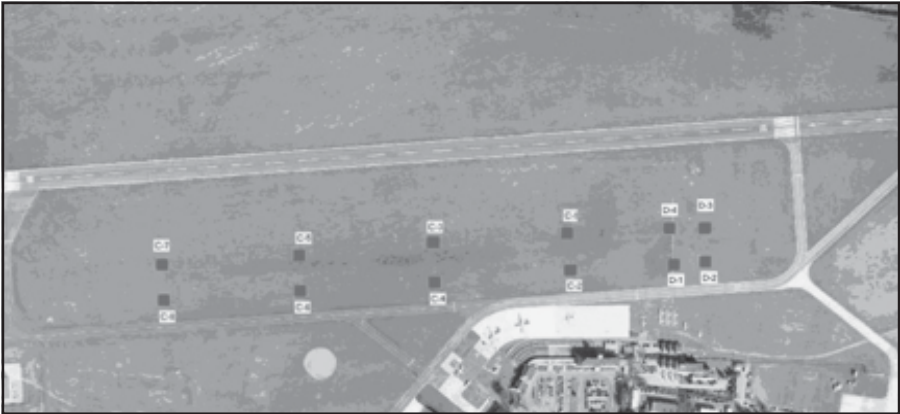
Figure 5. Installation of radar reflectors along grass runway 26 in Braunschweig, Germany, Corner reflectors C-1, ..., C-8 and Diplanes D-1, ..., D-4 with \alpha_1=2.3^\circ , \alpha_2=2.9^\circ , \alpha_3=3.5^\circ , \alpha_4=4.1^\circ supporting a precision straight-in landing with a 3.2^\circ nominal glide path.
