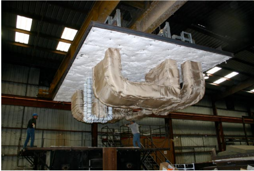
Figure 4 Hemyc fire barrier test on cable trays, pretest
