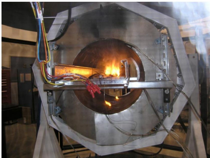
Figure 3 Small-scale CAROLFIRE test—two cables in a 30.48 cm (12 in.) cable tray
