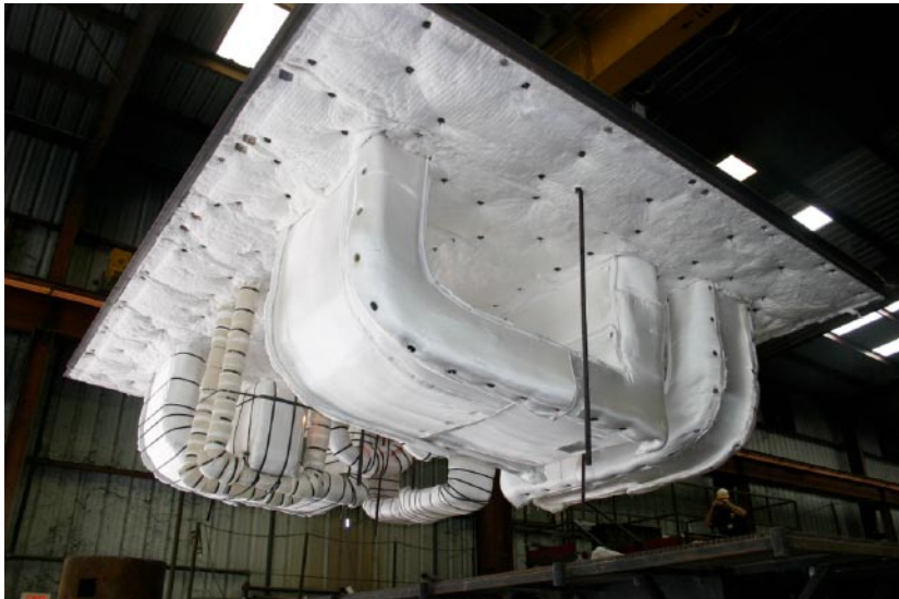
Figure 5 The same Hemyc fire barrier test on cable trays, posttest (note failed, glowing joints)
