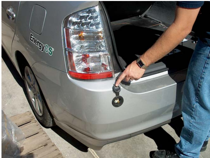
Figure 5-4. EnergyCS Level 1 charger plug-in receptacle.
