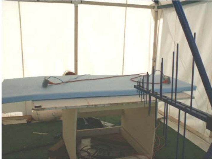
Yitran IT700 RE310 Radiated Emissions Photos Test Setup Continued
