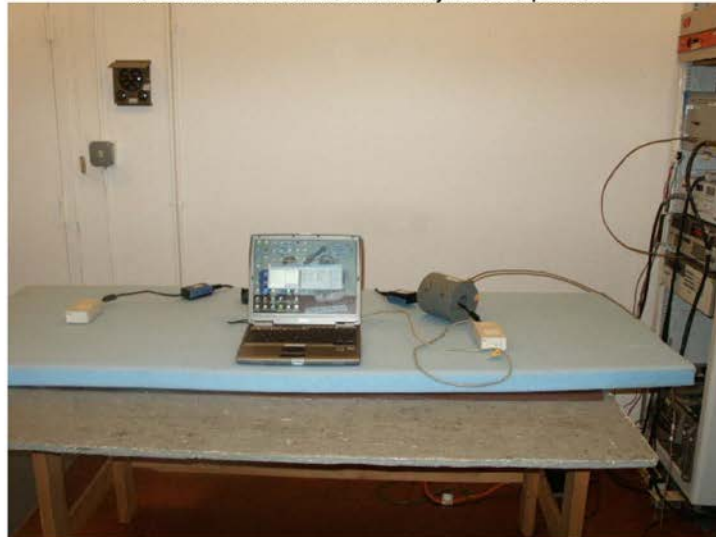
Yitran IT700 RI112 Radiated Immunity Test Setup Photos
