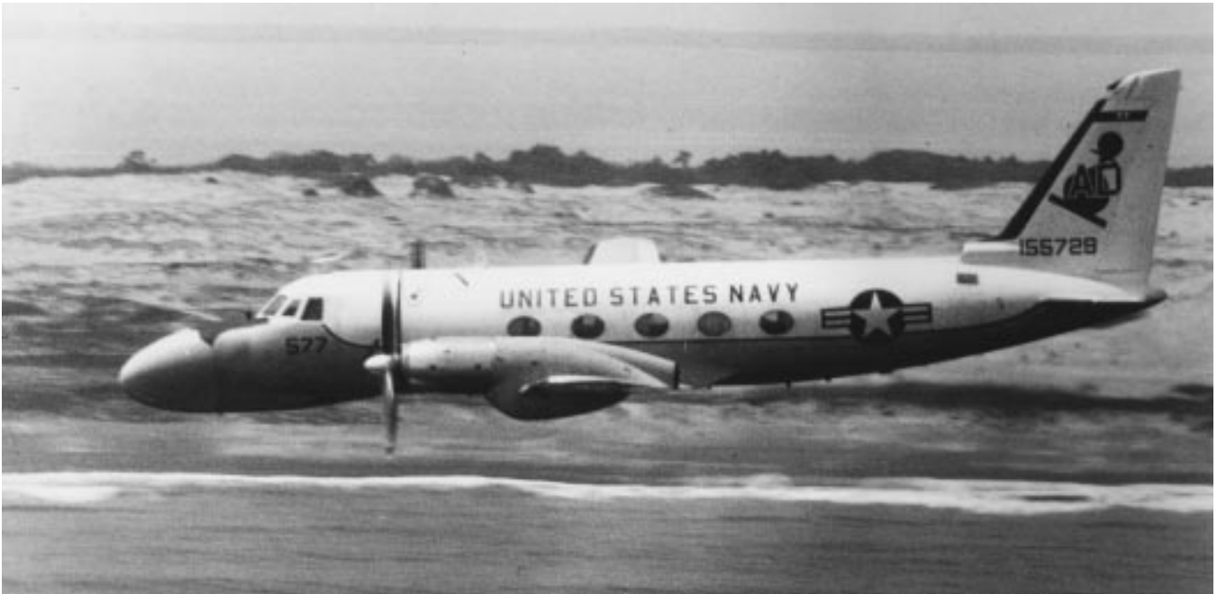
A squadron TC-4C Academe used to train Naval Flight Officers as bombardier navigators.
