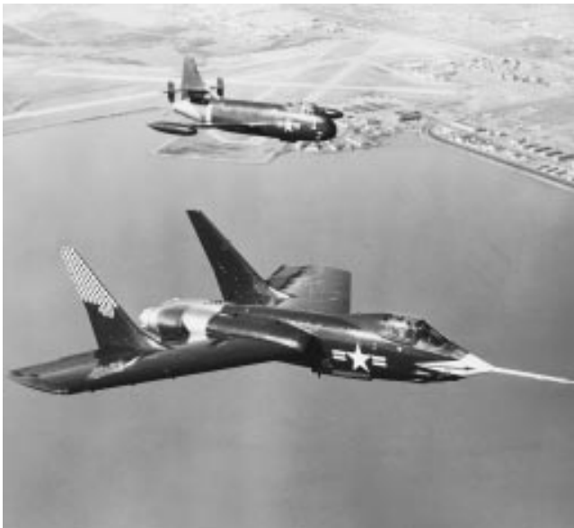
An F7U-3 Cutlass during a test flight, with an F6U-1 Pirate chase plane.
