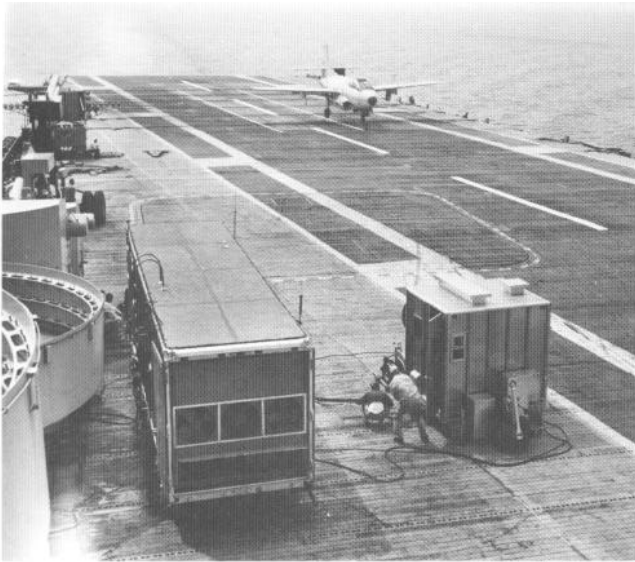
A Douglas F3D Skyknight lands aboard Antietam (CVS-36) off Pensacola, Fla., beginning the first shipboard tests of the automatic carrier landing system (ACLS).
